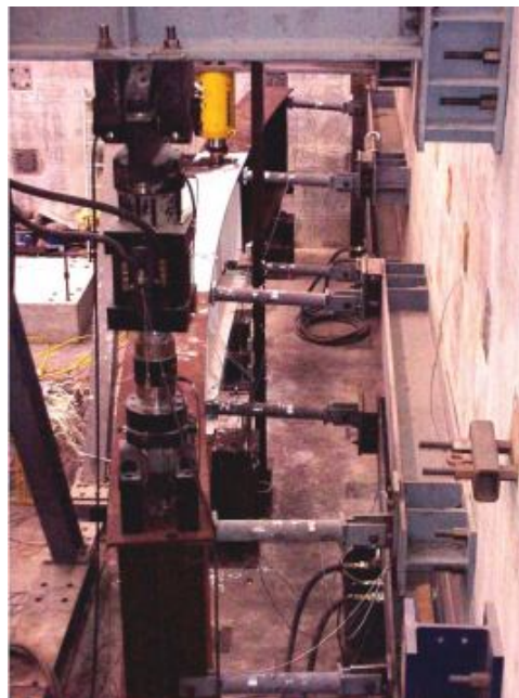
Figure 1: Tensile field in curved plate girder (Shanmugam, 2003)
